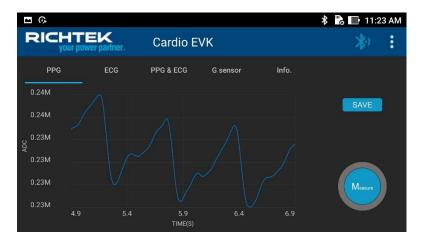
If the Red/IR LED was selected, two PPG data for both Red and IR LED will display the waveform on PPG Tab. (RED/IR LED method has different capability; i.e. SpO2 (Blood oxygen level))
