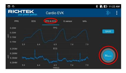
G sensor : To acquire the G-sensor value, click "G sensor" tab in the Cardio EVK first. Then press "Measure" to start the measurement. Shaking the EVB in different directions will produce below results. Press "Stop", once you finish the measurement.
