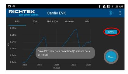
Measure : The "Measure" button is used to measure the PPG/ECG/PPG&ECG/G-sensor signal from Cardioid Pad device. During the data acquiring, the button will be changed to "Stop"
