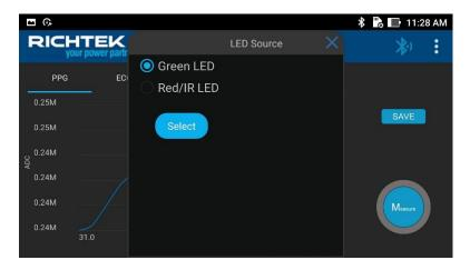
If the Green LED was selected, only one PPG data will display the waveform on PPG Tab.
