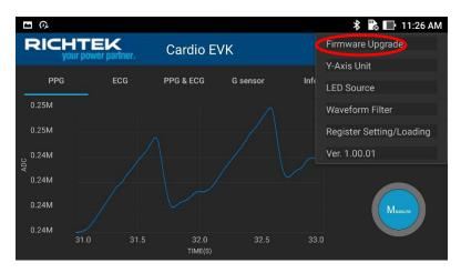
The battery voltage needs to be greater than 3.8V when FW upgrade.
