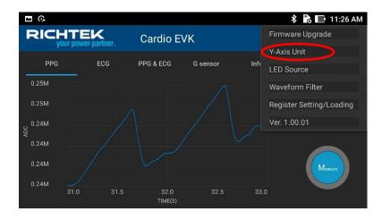
LED Source : Cardioid PAD provide the Green and the Red/IR LED sources for PPG measurement. This function can switch the LED source for PPG measurement.
