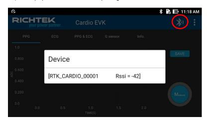
• After the Cardioid evaluation board BLE connection is successfully established, the "BLE ICON" will become blue and the main GUI will launch.
