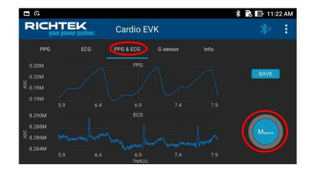
4. Check the measurement results. Press "SAVE" to store the measured data for analysis.
